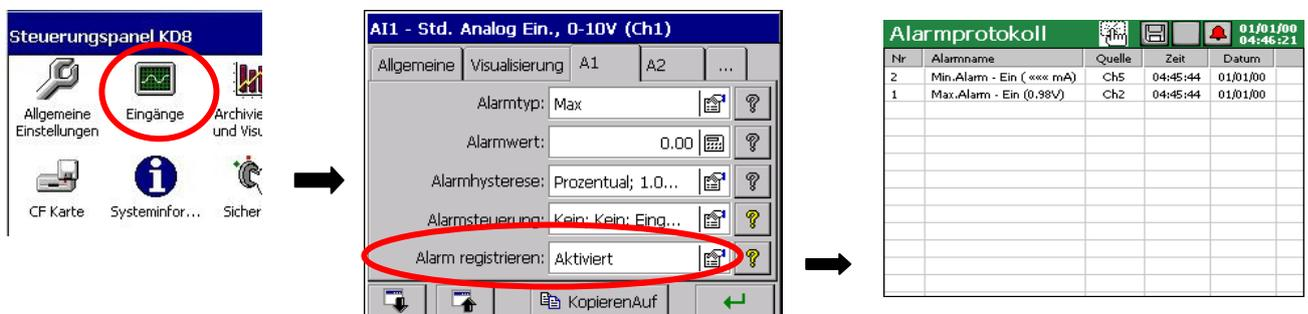
The image shows a sequence of three screenshots. The first is the 'Steuerungspanel KDB' main menu with 'Eingänge' circled in red. An arrow points to the second screenshot, 'A11 - Std. Analog Ein., 0-10V (Ch1)', where the 'A1' tab is selected and 'Alarm registrieren' is set to 'Aktiviert' (circled in red). A final arrow points to the third screenshot, 'Alarmprotokoll', which is a table showing two entries:
